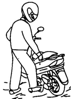
**CAUTION:** If you start your scooter while it is on its centre stand the auto choke may cause the clutch to engage and the rear wheel will start to spin. Take care to use the rear brake to stop the wheel spinning before taking it off its centre stand. Otherwise the scooter may lurch forward when the rear wheel suddenly comes in contact with the ground.
