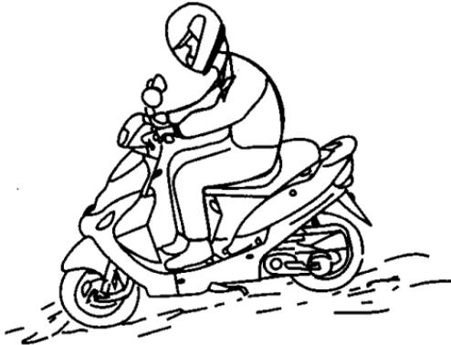
When travelling uphill the scooter will automatically increase the revs and decrease the speed, it will find the right loading on the belt drive to gain the maximum speed possible on any given grade.
